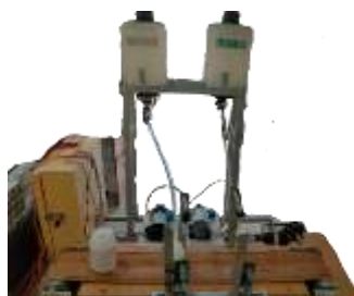
Figure 1: Automatic filling station having two units A and B
